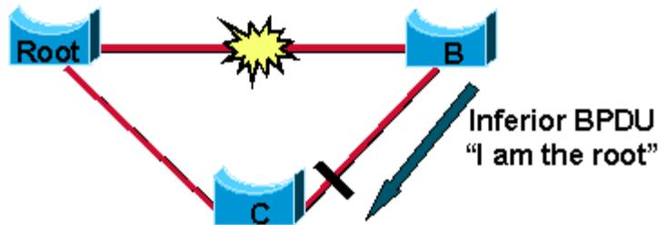
Because Bridge C still knows the root is alive and well, it immediately sends a BPDU to Bridge B that contains information about the root bridge. As a result, Bridge B does not send its own BPDUs and accepts the port that leads to Bridge C as the new root port.
