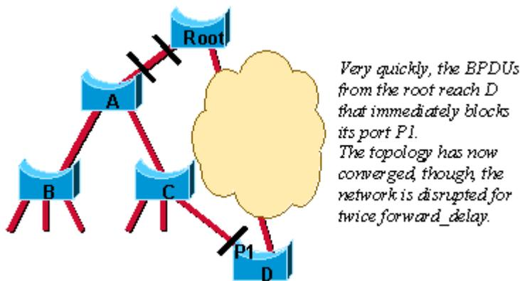
Spanning tree is very efficient in how it calculates the new topology of the network. The only problem now is that twice the forward delay must elapse before the link between the root and Bridge A eventually ends up in the forwarding state. This means 30 seconds of disruption of traffic (the entire A, B, and C part of the network is isolated) because the 802.1D algorithm lacks a feedback mechanism to clearly advertise that the network converges in a matter of seconds.
