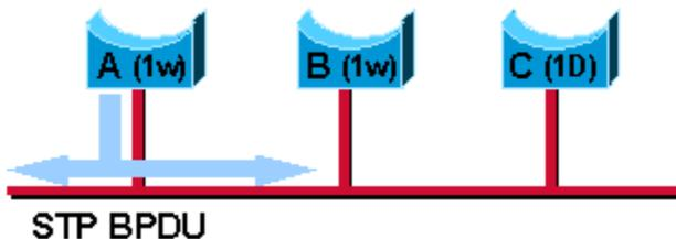
Notice in this particular case, if Bridge C is removed, Bridge A runs in STP mode on that port even though it is able to work more efficiently in RSTP mode with its unique neighbor B. This is because A does not know Bridge C is removed from the segment. For this particular (rare) case, user intervention is required in order to restart the protocol detection of the port manually.
