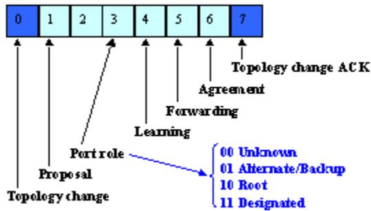
Another important change is that the RSTP BPDU is now of type 2, version 2. The implication is that legacy bridges must drop this new BPDU. This property makes it easy for a 802.1w bridge to detect legacy bridges connected to it.
