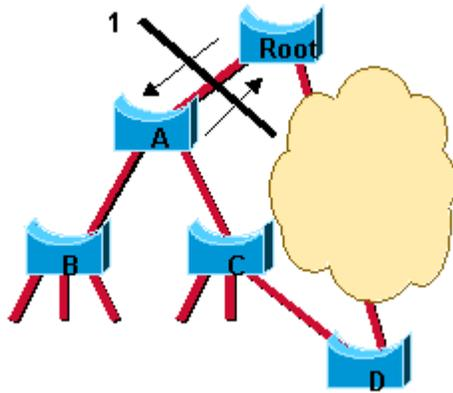
Once Switch A blocks its non-edge designated ports, the link between Switch A and the root is put in the forwarding state and you reach the situation:
