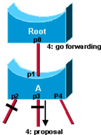
Once p0 receives that agreement, it can immediately transition to the forwarding state. This is step 4 of the preceding figure. Notice that port p3 is left in a designated discarding state after the sync. In step 4, that port is in the exact same situation as port p0 is in step 1. It then starts to propose to its neighbor, and attempts to quickly transition to the forwarding state.
