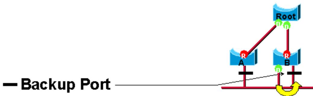
This distinction is already made internally within 802.1D. This is essentially how Cisco UplinkFast functions. The rationale is that an alternate port provides an alternate path to the root bridge and therefore can replace the root port if it fails. Of course, a backup port provides redundant connectivity to the same segment and cannot guarantee an alternate connectivity to the root bridge. Therefore, it is excluded from the uplink group.
